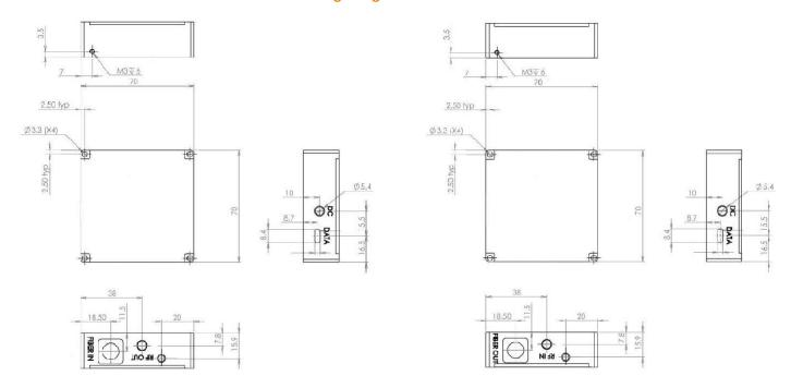
Connector: Positive center plug OD: 3.5mm, ID: 1.3mm, L: 9mm
